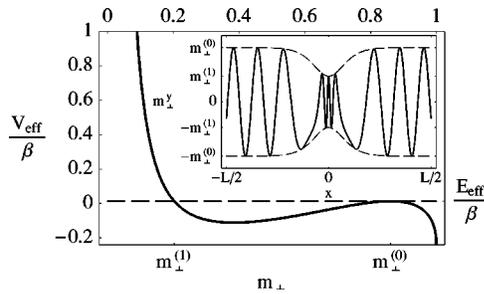
FIG. 3. Main Plot: Effective potential, Eq. (10b), for the mechanical analogy of the EL equations plotted for  $v=0.5$  and  $j=0.1$ . The physically stable configuration is the mechanically unstable point  $m_{\perp}^{(0)}$ . Inset: Schematic drawing of the saddle-point (bounce) solution—the dominant contribution to the transition probability.
