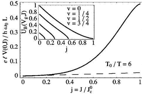
FIG. 2. Main Plot:  $IV$  curve for  $J < J_c(V_g)$ ,  $\rho_s^z = \rho_s^\perp$ ,  $V_g = 0$  and  $T_0/T = 6$ . Inset: Energy barrier for various gate voltages  $v = V_g/2\beta$ , with the barrier vanishing for  $v \rightarrow 1$ . Qualitatively similar curves are obtained for the full range  $0 \leq \rho_s^z/\rho_s^\perp \leq 1$ .
