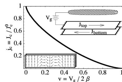
FIG. 1. Main Plot: Critical staggered current  $j_c$  as a function of gate voltage  $v$ . Upper Inset: Sample geometry considered in this work. Lower Inset: Pseudospin configuration of the  $2\pi$ -line soliton whose nucleation leads to staggered-current decay.
