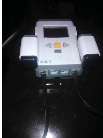
Figure 3.1: The Lego MINDSTORM NXT ® , configured with Hitechnic gyro and compass sensors
