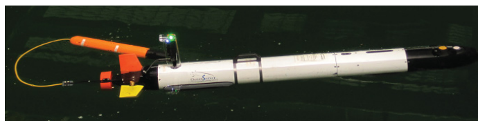
Figure 1.1: One of the DRDC Iver2 lightweight autonomous underwater vehicles. When submerged, the vehicle uses dead reckoning, incorporating DVL and compass input to maintain an estimate on current positioning between GPS fixes when surfaced.
