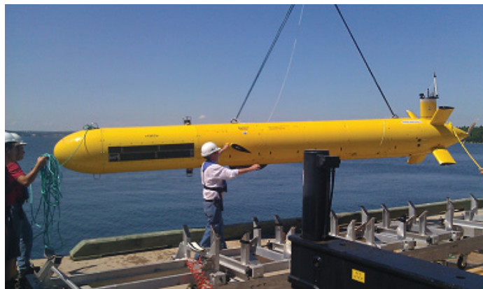
Figure 1.2: One of the DRDC Arctic Explorer autonomous underwater vehicles. When submerged, the vehicle uses an Inertial Navigation System to provide an estimate on current positioning between GPS fixes when surfaced.
